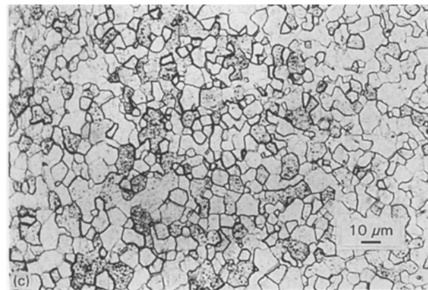
Figure 13 Recovered Ta jet fragment (a) showing essentially uniform cross-section microstructure (b) similar to forged copper (Fig. 4). (c) Shows magnified view of equiaxed grain structure.
